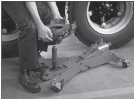
1. The clutch is loaded in a flat position with the Clutch Adapter's splined shaft in the upright position.
