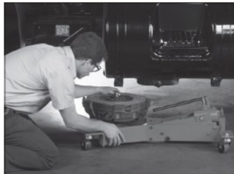
3. It's the only tool with a profile low enough (13") to allow the tool and the clutch to roll under the truck. The clutch can be loaded onto the Clutch Caddy next to the truck, not under it.
