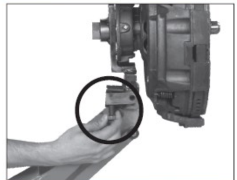
5. An adjustment bolt on the clutch holder assembly aligns the shaft with the angle of the engine. The end of the splined shaft is drilled and tapped for a slide hammer. This feature is useful when removing the splined shaft from the clutch.
