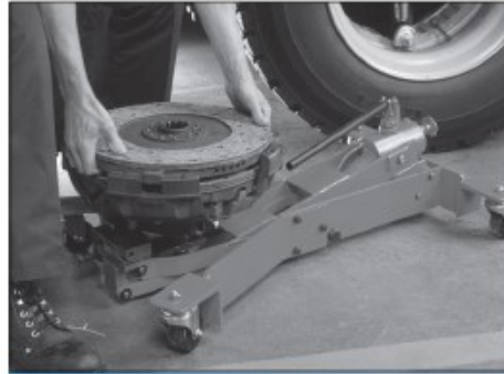
2. Clutches can be assembled or disassembled piece-by-piece to avoid lifting the complete hard-to-handle component.
