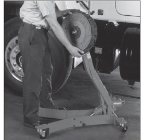
4. The clutch can be raised to a height of 39". The Caddy's ability to swivel 360° minimizes alignment problems.
